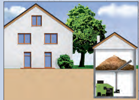
Example: silo delivery from a chip silo using a silo feeding system
